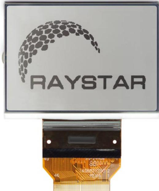
**Tape automated bonding (TAB) LC modules** are available in resolutions of 128 x 64 to 320 x 240 pixels. The controller is mounted on a TCP (tape carrier package). The TCP is connected with the ITO contacts on the LCD. TAB modules are extremely thin and require little space as the TCP can be folded down to the back of the LC module.
