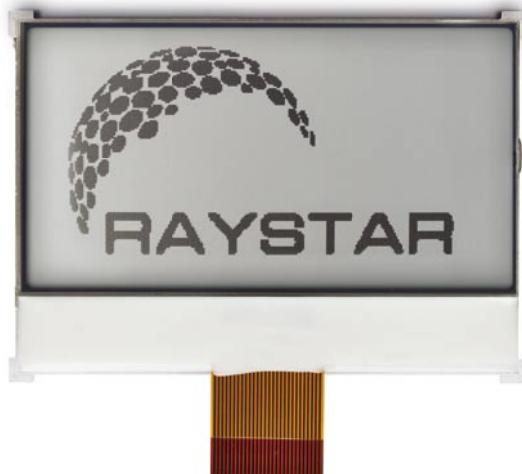
**Chip on glass (COG) LC modules** are available as standard products in resolutions of 16 x 2 characters to 320 x 240 pixels. The controller is bonded to the LCD glass. The advantages of COG compared to COB modules are a lower construction height and weight and a better shock resistance.
